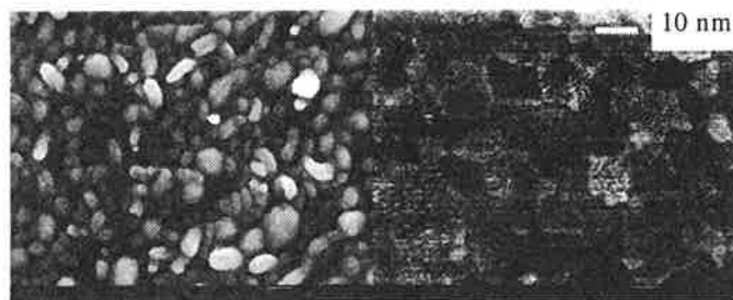
(a) Bombardment by recoiled Ar (b) Suppressed bombardment Fig. 2. SEM images of typical ITO films deposited by Ion beam Sputtering IBS. (Ar gas flow: 2 sccm, \text{O}_2 gas flow: 0.5 sccm)
