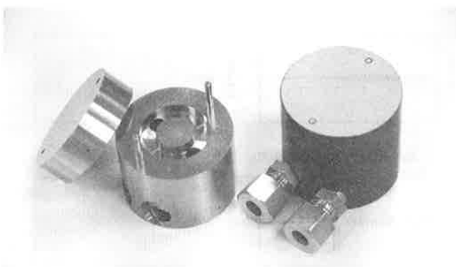
Fig.1 Appearance and internal structure of the mold used for the heat cycle test.
