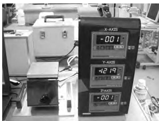
Fig.1 Portable tactile meter (Heidon Type 33, SHINTO Scientific Co. Ltd.)
