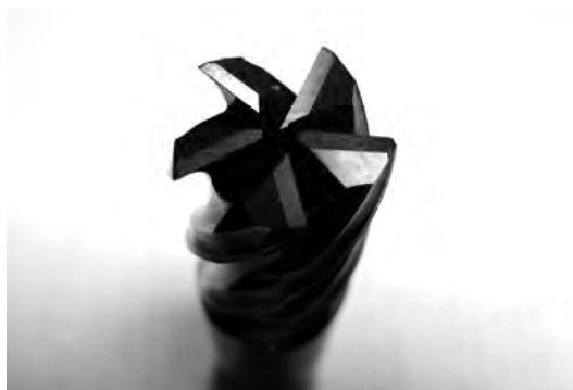
Fig. 1 View of an endmill used in the experiments.
