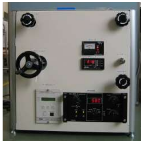
Fig.1 The desktop type RIE system.
