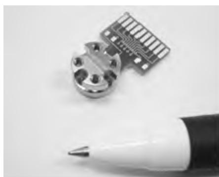
Fig. 2 Piezoresistive 3-Axis Force Sensor
