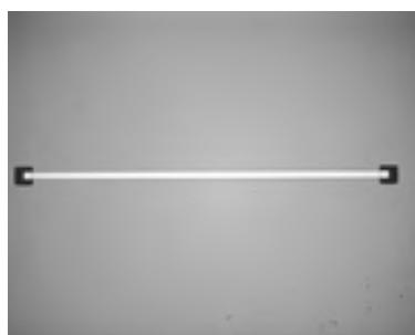
Fig. 1 Piezoresistive element
