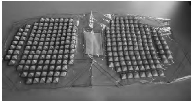
Fig.5 Pyramid piles adhered to insides of bag
