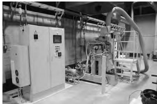
Fig. 1 Cellulose mixing-plastication molding machine
