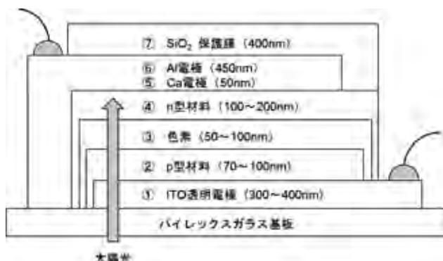
Fig. 1 Structure of organic thin-film solar cell.
