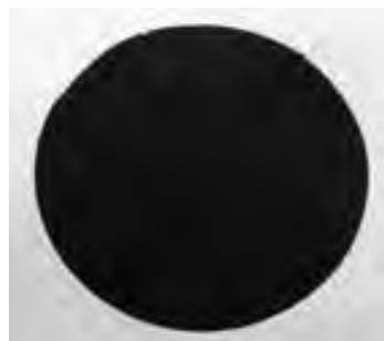
Fig. 2 Conductive CNF sheet.
