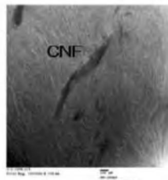
Fig. 1 TEM image of CNF/PP composite.
