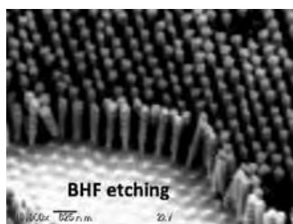
Fig.4 Etched  $\text{SiO}_2$  nano-pillar
