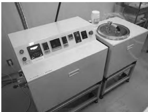
Fig. 1 Parylene coating process system
