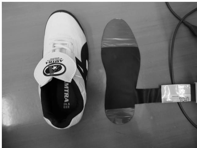
Fig. 1 Shoe and the pressure sensor
