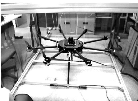
Fig. 1 Multi-copter for upper inspection with 8 rotor arms
