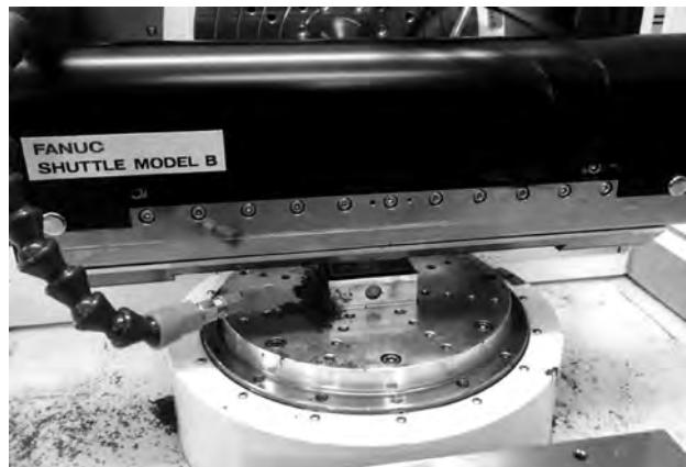
Fig. 1 Experimental setup for machining nickel phosphorus layer using ultra-precision cutting machine with shuttle unit
