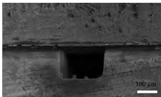
Fig. 1 Cross-sectional view of PFA microfluidic chip
