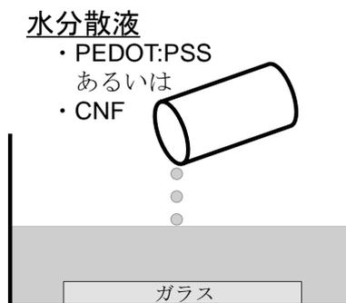
Fig. 1 Schematic diagram of casting method
