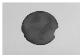
Fig. 2 Pressure sintered cathode substrate
